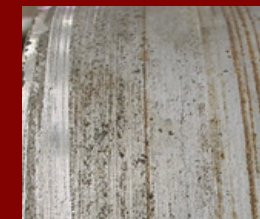
Look familiar? Typical flaking and corrosion on chrome-plated glue roll; scoring on doctor roll.
