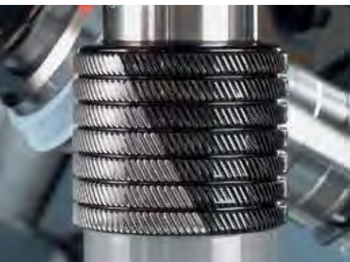
Grinding of hardened gears
