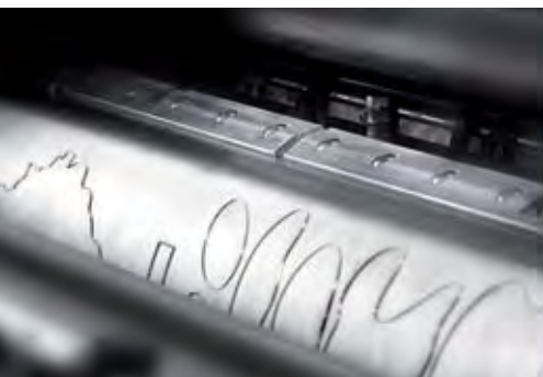
The manageable clamping with rails system from Spilker for a secure hold and an easy flexible die fitting.
