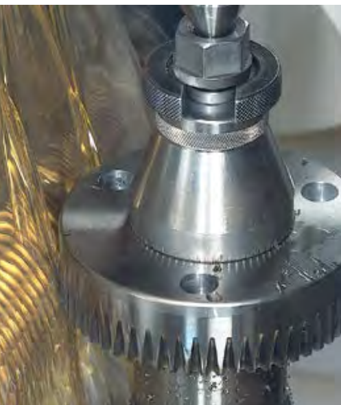
Gearing at the hobbing process
